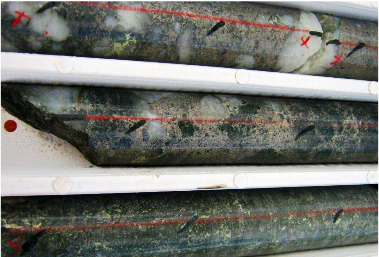
Figure 1. Photo of nickel-bearing breccia sulphide and disseminated chalcopyrite in SYMD0006, Inky prospect, Youanmi.
